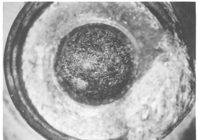
FIG. 3—Fitting (23A) from the Beechcraft's engine fuel line, viewed from above, showing the mass of stellate trichomes and an amorphous matrix within the orifice, and melted aluminum residue at the face (lower right).
